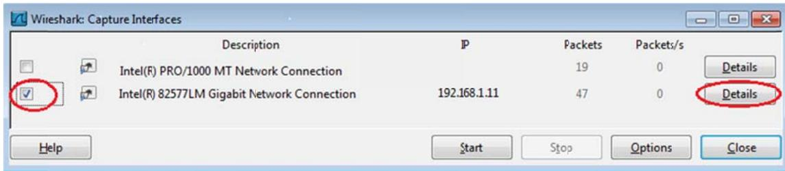
**Note:** If multiple interfaces are listed and you are unsure which interface to check, click the **Details** button, and then click the **802.3 (Ethernet)** tab. Verify that the MAC address matches what you noted in Step 1b. Close the Interface Details window after verifying the correct interface.
