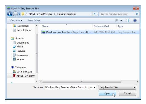
Locate and open the "Transfer data files" folder saved on the USB flash drive, select the **Windows Easy Transfer – Item from old ...** file, and then click **Open**.
