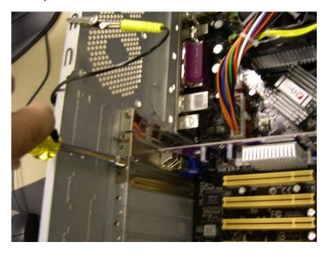
Make sure the wireless NIC is properly lined up with the slot. Push down gently on the wireless NIC.
